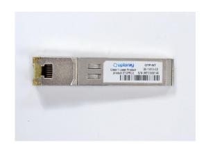
The OTP-100T1-I Copper SFP transceiver is high performance, cost effective module compliant with the 100Mbps Fast Ethernet and 100BASE-F standards as specified in IEEE 802.3, which supporting 100Mbps datarate up to 100 meters reach over UTP cable. It can auto-negotiate optimal network speed, and supports 100 Mbps full duplex data-links with 3-level Pulse Amplitude Modulation (PAM) signals.
